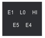
Make fault judgment and take corresponding actions after starting up. Regardless of the state, the fault is executed first and the fault code is displayed on the interface. If there is a fault in the sub-menu operation, immediately return to this interface display fault (including defrosting state). (the fault is judged when the pump works, and the fault is displayed as usual, but the pump needs to complete the water pumping this time). Multiple faults can be displayed at the same time.
